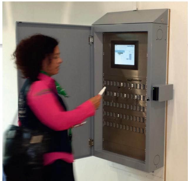
KeyConductor keeps a full audit trail of collected and returned keys, which can always be retrieved on the display, or which can be downloaded on a USB stick. Furthermore, the barcode version comes standard with a door and electronic lock.
